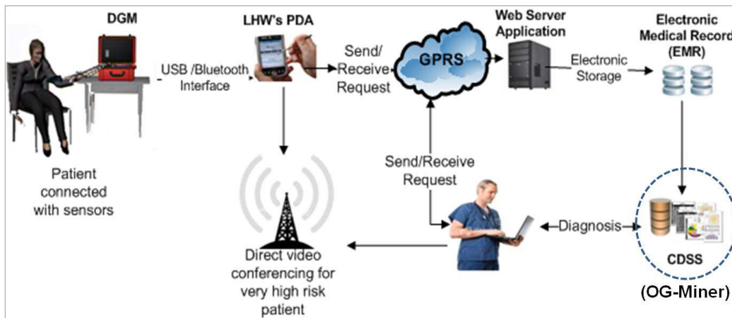
Fig. 1. Work flow of information in our project of Remote Patient Monitoring System
