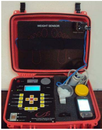
Fig. 16. LHW's Sensor box for measuring vitals
